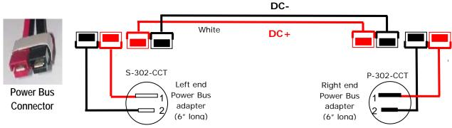
Note in the diagram that the solid color represents the tongue while the white space represents the contact opening of the housing. Using this convention you can determine we have red on the left of the DC power bus and black on the right.
