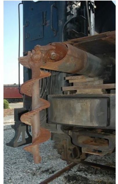
The stoker screw on 611's tender.
