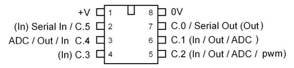
Note the labeling of pins as C.0, C.1 etc. For the 8 pin picaxes, it is not necessary to use the C. prefix - and just using 0, 1 etc will work OK.
