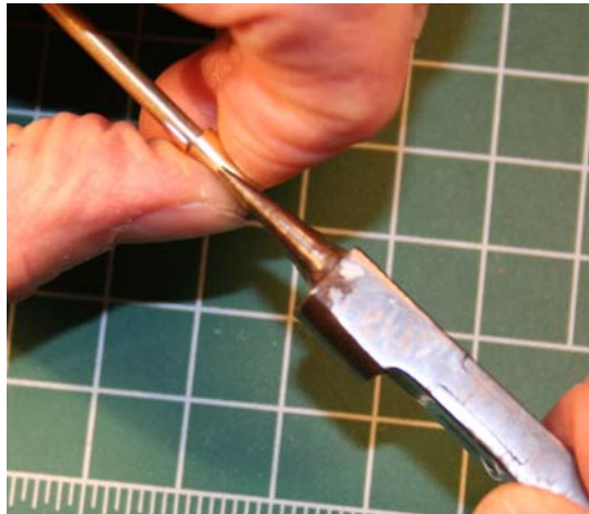
Figure 5: Bending the Target Housing using a brass tube for a form and round-tip needle nose pliers
