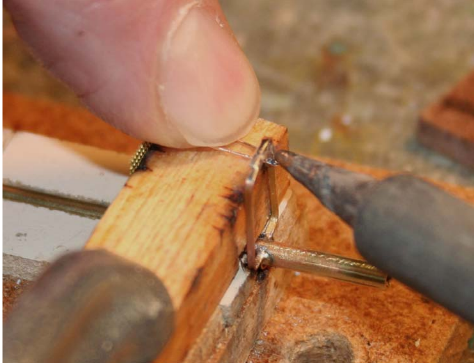
Figure 15. Soldering one vertical handrail
