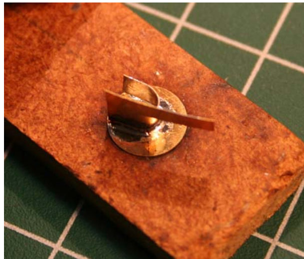
Figure 7: Soldered Target assembly
