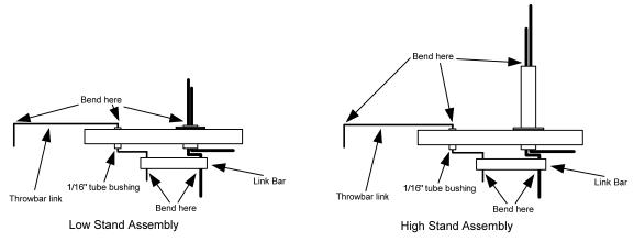
Figure 5: Final assembly, Side view (Stops are not shown)
