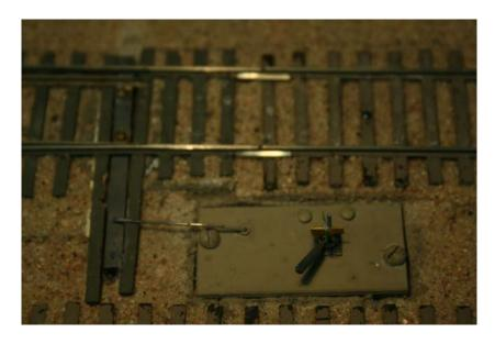
Figure 9: Installed Low Ground Throw
