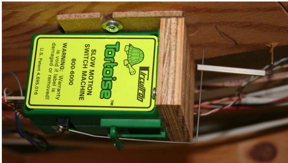
Figure 4: Tortoise Motor Horizontal Assembly Bottom View
