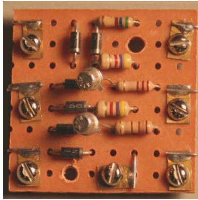
Figure 19 Type D Display Module Component Front Layout
