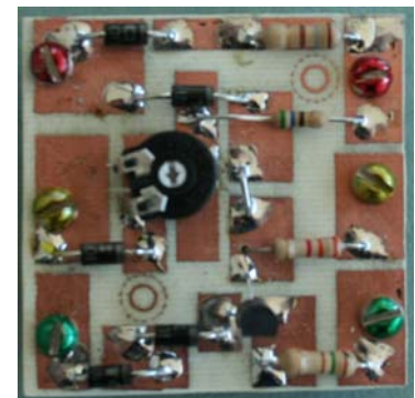
Figure 24 Type SA Display Module Printed Circuit Component Layout
