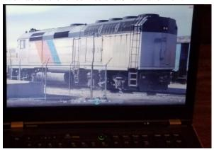
Larry Stephens' video of a GP40FH-2. Created from an Amtrak GP40. It uses a frame of a GP40
