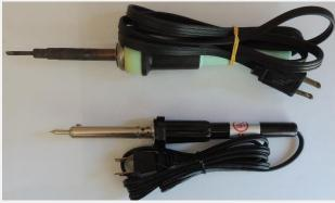
Various manufacturers have made pointed tip soldering irons (bottom of photo above) that are held in with a set screw. My opinion of these soldering irons are that they are prone to poor heat transfer. Enter the 21st Century. With its slowly shrinking electronics, these irons are not the best for microelectronics.
