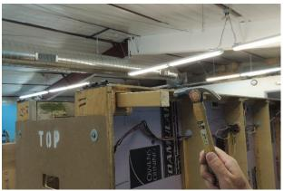
A  $1\frac{1}{2}$ "x $1\frac{1}{2}$ "x1" block of wood is inserted and is driven in a precise distance.
