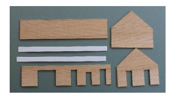
Because I was joining two dissimilar materials, I braced the interior with matboard after cutting out the door and window openings on the matboard. I cemented the wood siding and the matboard together with contact cement, clamping everything together so that they would remain flat. Next, I sealed all parts with sanding sealer, inside and out, to prevent warping when the parts were painted:
