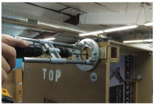
Two 1/4" holes are drilled into the leg pocket through the block of wood that was inserted into the pocket to hold two dowels.
