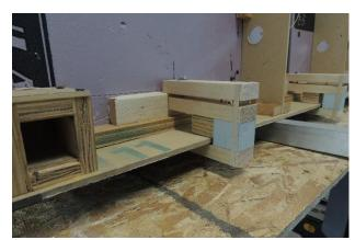
A homemade clamp (eight of them, four on the top and four on the bottom) is used to hold a 1x2 block of wood to the module frame and the foam base of the module.
