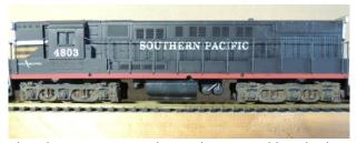
This close-up picture shows the painted handrails, the addition of a small round tank to the left underframe (which Athearn had omitted) and piping added to the air tanks. The trucks were weathered to indicate usage and to highlight details. Lastly, Larry had to remove the casting ridge from fuel tank.
