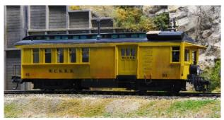
Dennis Hagen took an old HO scale Atlas RS-3 and regauged the trucks to make it run on Sn3 track. Then he simply threw away the diesel shell and scratch built the doodlebug shell from styrene and attached it to the diesel chassis. Even though it is no longer a diesel locomotive he thought that it might make an interesting diesel into a non-diesel conversion project to briefly describe.
