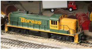
Stu Jones showed his Boreas and Saguache Railroad RS3. He stated that the ALCO RS3 is a 1,600 hp. locomotive that was manufactured by the American Locomotive Company (ALCO) and ALCO's subsidiary Montreal Locomotive Works (MLW) from May 1950 to August 1956. It has a single, 12 cylinder, model 244 prime mover. 1,418 were produced: 1,265 for American railroads, 98 for Canadian railroads, 48 for Brazilian railroads and 7 for Mexican railroads.
