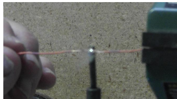
Place iron under wire and apply evenly.
