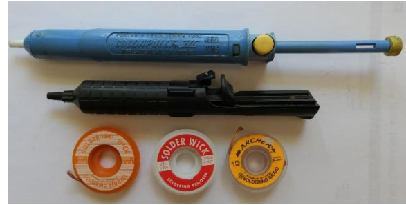
Removing solder tools: vacuum pullers and solder wick.
