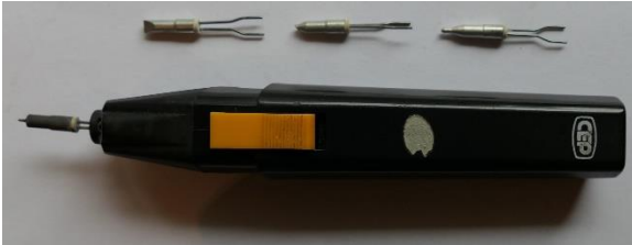
The soldering iron I use most is the Iso-Tip. It heats up quickly and has no cord in the way. It also has some of the smallest tips available. It is capable of soldering feeder wire to rail.
