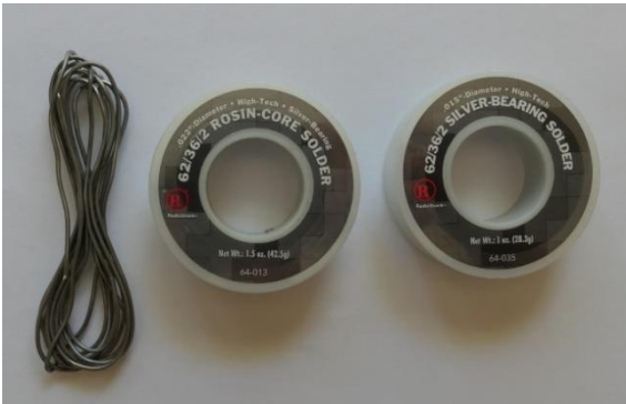
Three of the most common solder sizes left to right. 0.047 is a good general purpose solder. 0.022 works great for small wires such as feeders. 0.015 works great for DCC wires and SMD devices.
