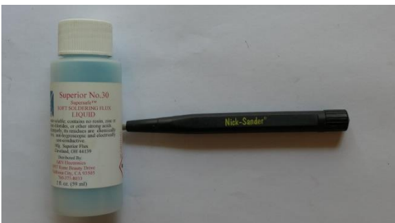
Safe flux and a fiberglass surface cleaner. Safe Flux works best on tinned wire and very clean copper. Fiberglass cleaner is used to clean rail and such prior to applying flux. For harder to solder items, use a rosin flux.
