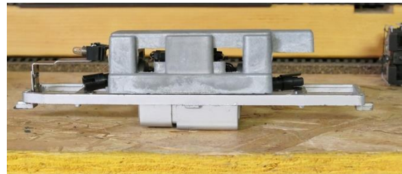
Athearn's F7 could be purchased as Super Powered. The weight allowed it to pull longer trains.
