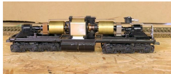
Athearn's latest motor in the Blue Box series. This motor is the one to use for DCC.
