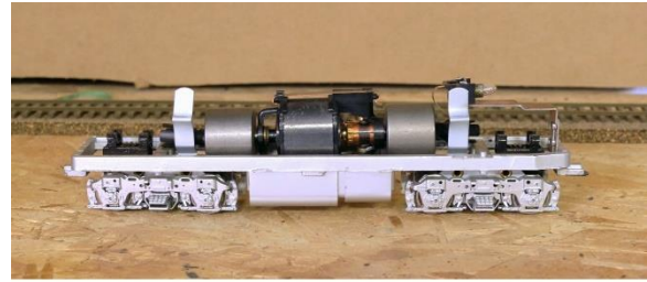
Athearn's next motor and it was gear driven. This motor is not recommended for DCC.
