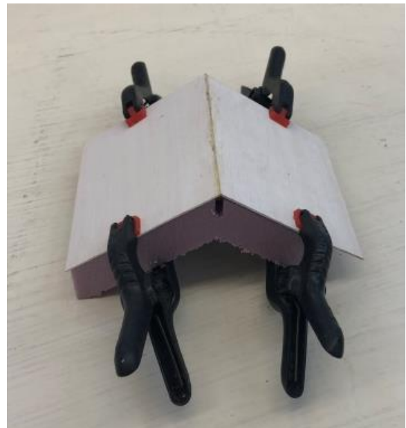
Roof boards in clamps, with formers, part one.
