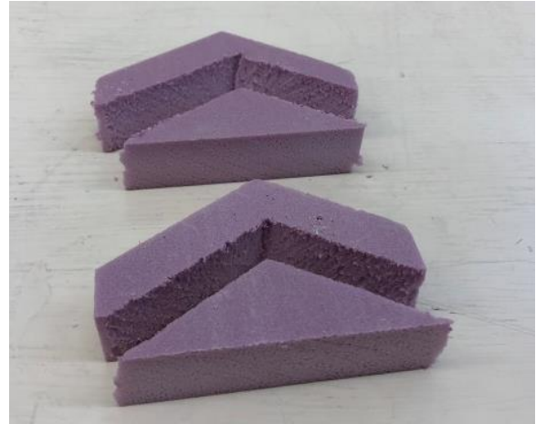
Foam formers to clamp the roof angle. No cost.
