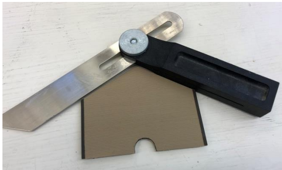
Sliding angle bracket to establish the roof angle. I did not have the adjustable clamp that Stuart spoke of a couple of meeting ago.
