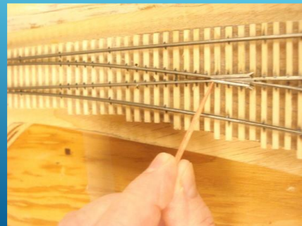
LOCATE CRITICAL POINT WHERE CLOSER RAIL BENDS TO BECOME WING RAIL
