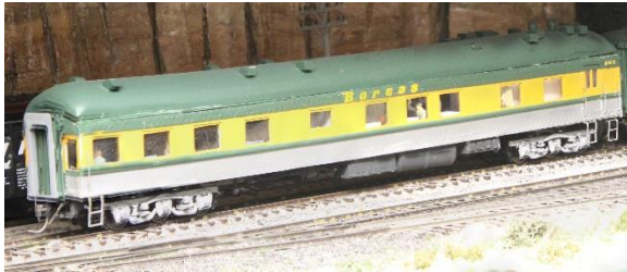
A scratchbuilt Diner-Lounge car using drawings for a Walther's-produced car in the 1940s (long out of production). It was designed for mid-train use, but the rear windows made it suitable as an observation car when used as the last car on a train
