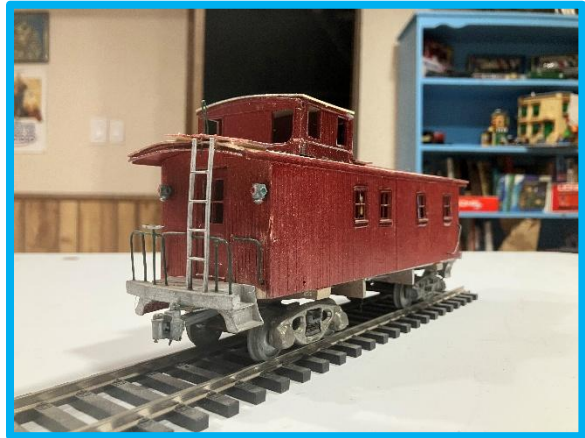
"In the 1950's my grandfather, Ed Keiss, purchased some trucks and couplers. He made an additional two truck side frames from scratch. In the 1990's he built this O scale Santa Fe caboose from an Ambroid kit to put them on". John Keiss
