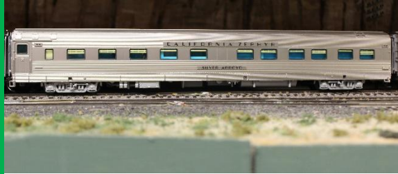
Budd 10-6 Sleeper 10 single bedrooms and 6 double bedrooms: 22 passengers Operated on Denver and California Zephyrs and other railroads
