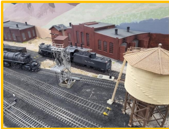
On the right is the turntable water tank. To the left, is the water column for both the inbound (stop #3) and outbound (stop #1) turntable tracks. In front of #3618 is stop # 2 on the inbound track, the ashpit. The ashes are picked up in a bucket and conveyed to the tower which dumps the ashes into a gondola that would be positioned on the track in front of the tower.
