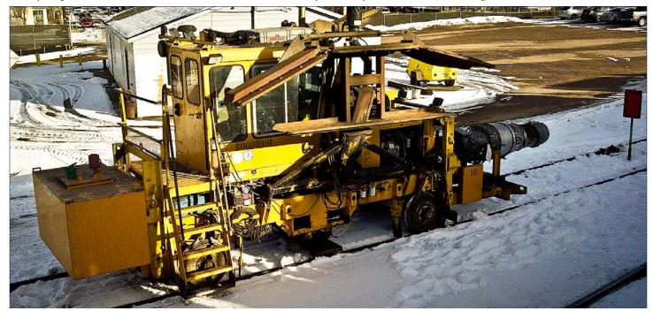
Tim Harkey couldn't bring his exhibit; that's because it is real. This is a snow blower on the BNSF. Basically it's a jet engine that can be pointed down and to the left and right. The exhaust from the engine melts and blows away the snow, along with loose bal-
