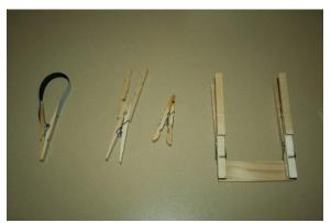
The clamp on the right is made from two extended clamps glued to a piece of plywood. With the plywood clamped in a vise, the long ends can secure a model for painting. Clothespins can also be notched on the clamping end to hold small parts or figures for painting.
