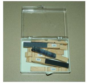
Larry's designs don't just end with clamps, however. He also takes pieces of disassembled clothespins and converts them into sanding sticks. The figure above shows sticks with various grades of sandpaper attached with rubber cement and labeled with the grit grades. He suggested buying a variety pack of sandpaper to obtain the various grades at the lowest price. He also suggested that we buy our own clothespins rather than liberate them from laundry duty to preserve domestic harmony.
