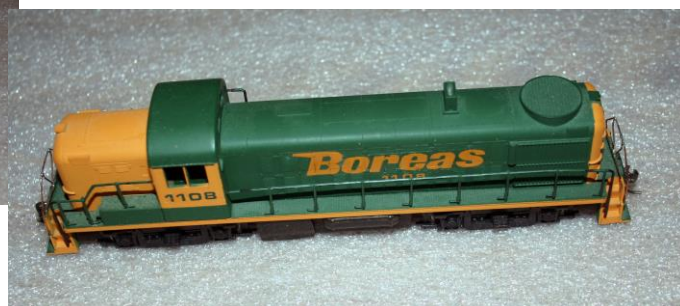
Stu Jones brought an Alco RS-3 road switcher lettered for his Boreas & Saguache Railroad. This originated as a Model Die Casting kit. At some time the end handrails were broken, so Stu replaced them with soldered brass replicas. The crew evidently keeps this locomotive very clean.
