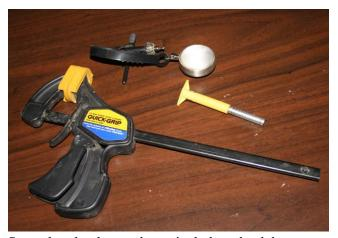
Several tools, shown above, include a chuck key attached to a retractable cord. This ensures that the key will always be within easy reach when it is needed while the retraction mechanism remains firmly attached to the user. Otherwise those pesky keys always seem to get misplaced. The second tool is a depth gauge used to determine if the hole being drilled is deep enough. The third tool is an ordinary friction clamp useful for securing the workpiece to be drilled.
