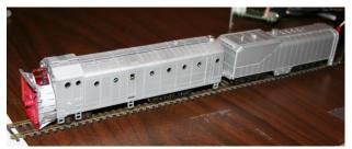
Larry Stevens displayed this Athearn HO scale rotary plow. The blades on his model actually spin, powered by a small motor that is controlled remotely through a decoder. He demonstrated that the blades will spin in either direction, depending on which side the operator wants to throw the snow. The blades also spin up and down slowly in a prototypical fashion
