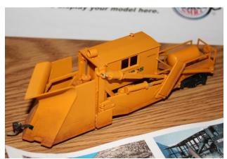
Stu Jones displayed this HO scale model of a Jordan Spreader, offered by Walthers about ten years ago. Spreaders were the preferred method for moving snow because they could push it far away from the track. Spreaders were also used for various duties besides moving snow including mining operations to move rock and gravel away from the track.
