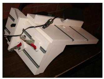
This apparatus is a drill press table for holding workpieces firmly in place. The moveable clamps attached to the tracks permit the work to be positioned for optimal effectiveness. This device is particularly useful for end-boring.
