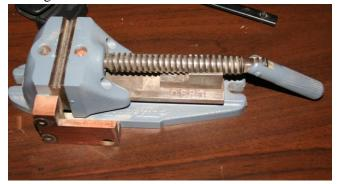
The tool shown above is a clamp for holding materials to be drilled. What is useful is that the screw can be lifted up to allow quick positioning of the jaws, then lowered and tightened to firmly hold the material. The notches at the end can be used to attach the clamp to the drill press base.
