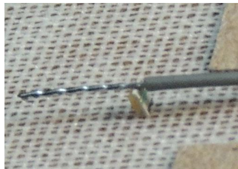
Figure 4: A Wire Positioned for Soldering. Larry uses decoder wire of the appropriate color for this application
