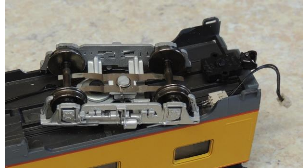
Figure 8: Axel wipers for electrical pickup
