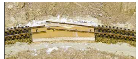
Quarter-inch Luan roadbed replaces the original cork roadbed where the rails in the flex track had kinked. You can see how the rails resist curving and want to be straight.
