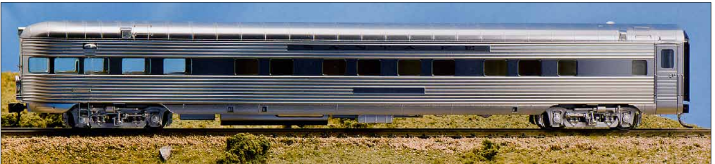
Getting the stainless steel look in two different ways is demonstrated by the new "plated" AT&SF tail car (above) and by using real foil for the fluting on a kit-bashed D&RG combine (below). Both cars belong to Bill Johnson.
