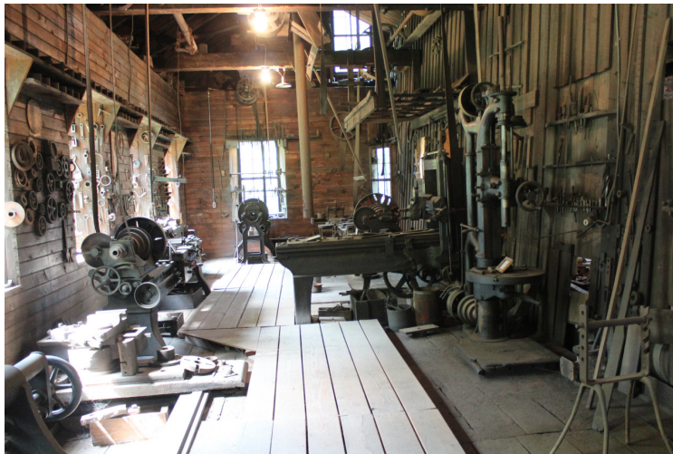
Partial view of the interior of Keystone Foundry, Hopewell, PA. Note overhead belt and pulley system. Dies, patterns, templates and forges are all in place. Knob & tube wiring and knife switches are also visible .
