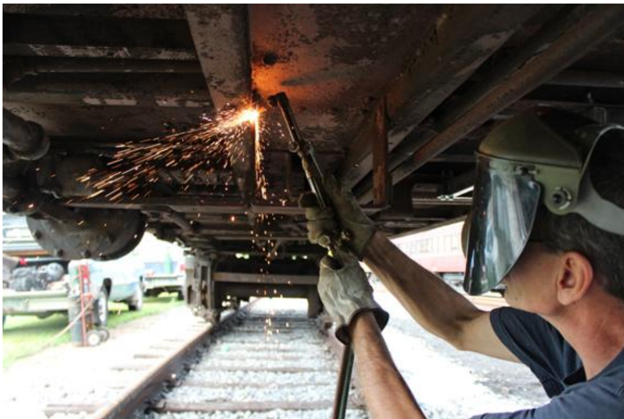
Replacing airbrake valves on Chapter Coaches.
