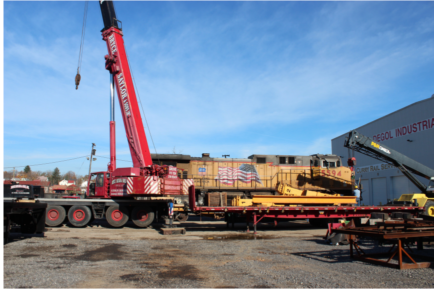
Preparations to life UP 5594 from a rail flat car onto timbers for car-body rehabilitation. The trucks/traction motors were on a separate carrier.
