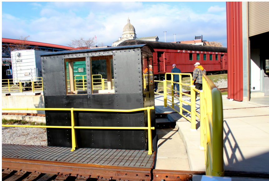
Turntable control unit, formerly installed on the PRR's East Altoona Roundhouse pre-1968. Fully restored. David Seidel photo
