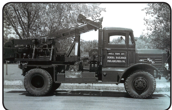
FWD Auger truck of the PRR used to set poles to electrify lines
