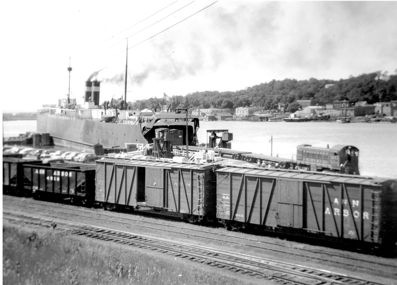
Ann Arbor No. 6 is being loaded at the west slip at Boat Landing in this mid-1950's view. Two 7400-series boxcars are coupled to a boat coaling hopper in the foreground.
