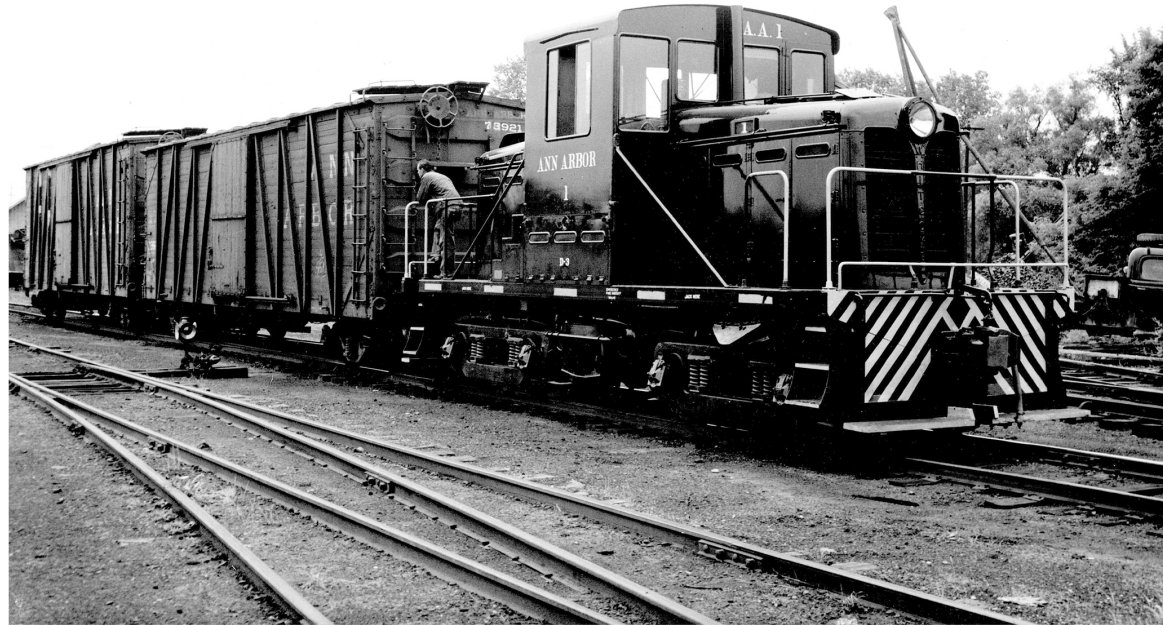
The difference in height between the 9' 73750-series and 10' 74000-series cars is evident in this 1955 Jim Shaw photo taken at Owosso.
