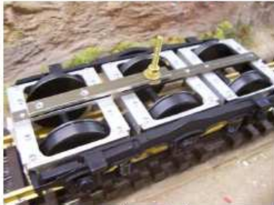
Motor block with Bigger wheels fitted, PA-1 side frames, cut and reworked.
