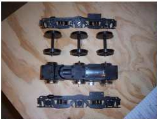
Removed the standard wheels, replaced them with bigger wheels.
