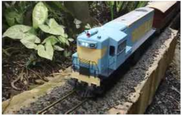
The model of this Queensland Railways Loco uses a USA Trains SD-40 motor block.
