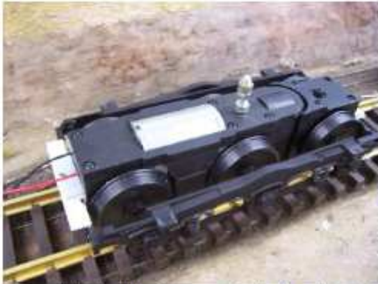
Motor block with Bigger wheels fitted, PA-1 side frames, cut and reworked.
