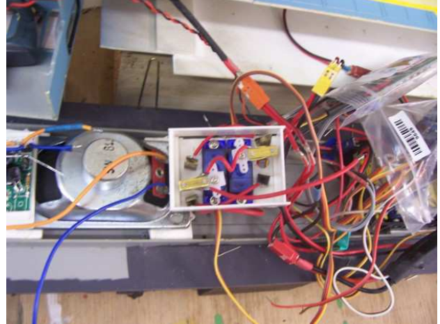
Switching mechanism driven by 2 mini servos.
