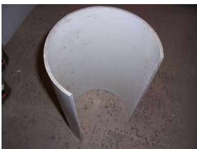
250mm diam Plastic pipe "slit" to width to be glued between "Hood" sides
