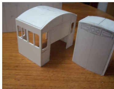
250mm diam Plastic pipe "slit" to width to be glued between "Hood" sides
