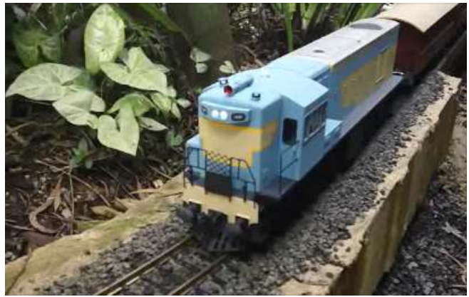
The model of this Queensland Railways Loco uses USA Trains SD-40 motor blocks.
