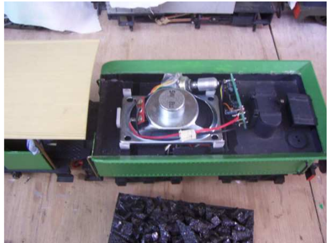
Two sound systems for three sounds are installed in the Tender; Chuff below, Pump & Whistle above.
