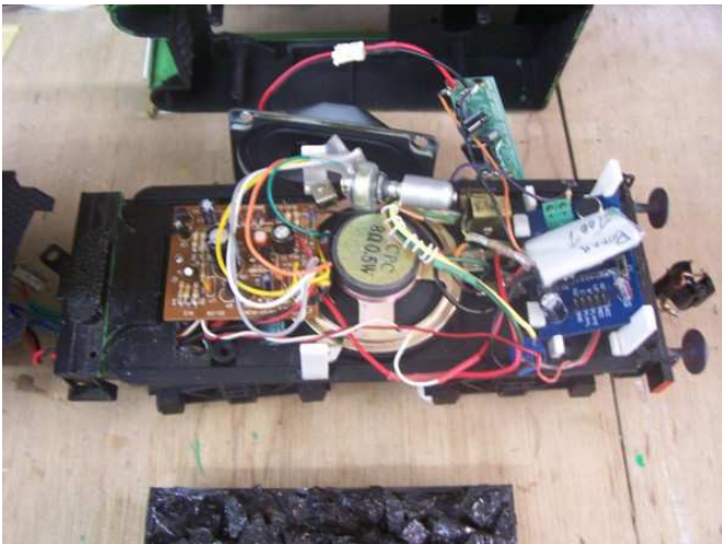
Two sound systems for three sounds are installed in the Tender; Chuff below, Pump & Whistle above.
