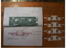
It is built on an Aristo-Craft Motor Block. The bogie frames are flimsy yet the Motor Block. Four (4) layers of 2.0mm styrene were temporarily glued together, then fritted out. Then frame layers are added, next springs, bolster end, journals & bolts, nut details were added.
