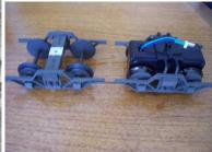
The truck or bogie frames ready for paint, the front bogie is an idler (un-powered).
