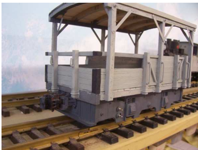
First coat of paint, thin washes of sooty black will bring out details, dry brush of white for highlights.
