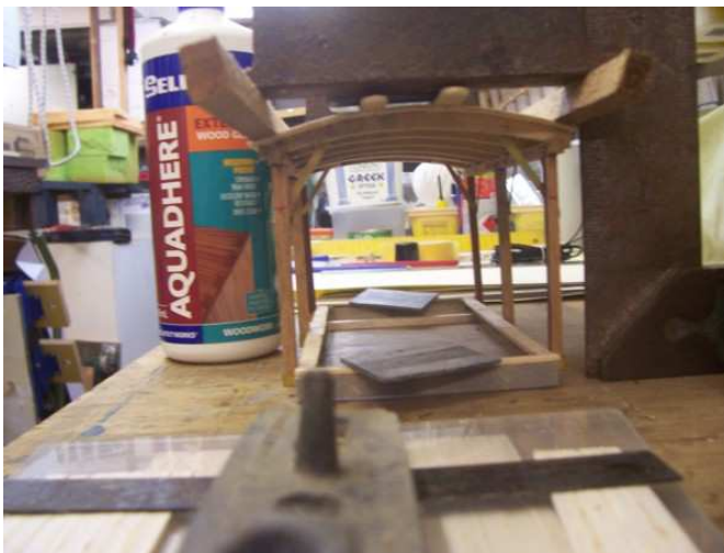
Sides and ends 7 plank 'fences' are glued and drying, roof arc sub strata is glued pressed and setting.
