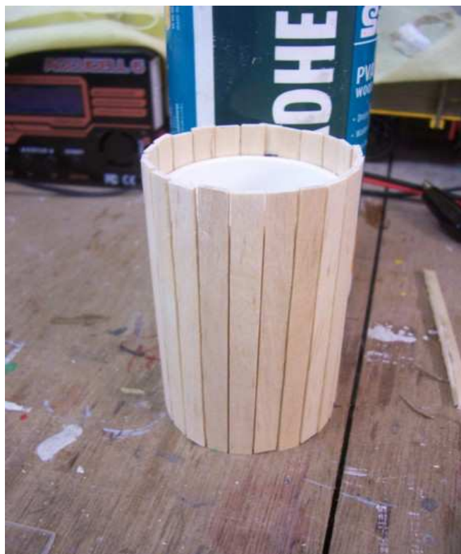
The vertical boiler is 40mm N.B. PVC pipe.
