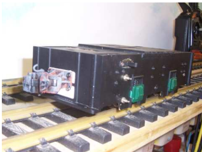
End plate, infills to accept KADEE # 905 couplers. Couplers fitted and ready to start painting the Base.
