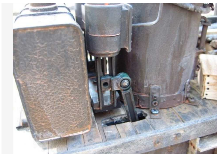
Close up of water tank, engine and the vertical boiler. stock.
