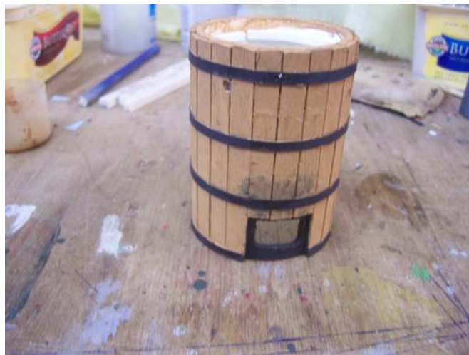
Boiler lagging & barrel bands, holes for feed water, steam pipe, water gauge, wash out plug & fire door.
