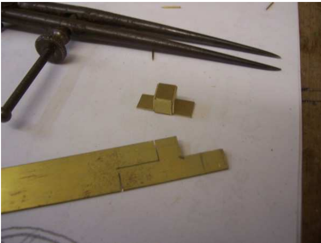
Sill sockets for the posts 0.5mm x 10mm brass cut to and folded and drilled for pins to attach to sill plate.
