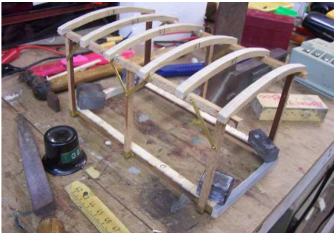
Roof arc rafters were fretted from 7mm thick 7 ply.
