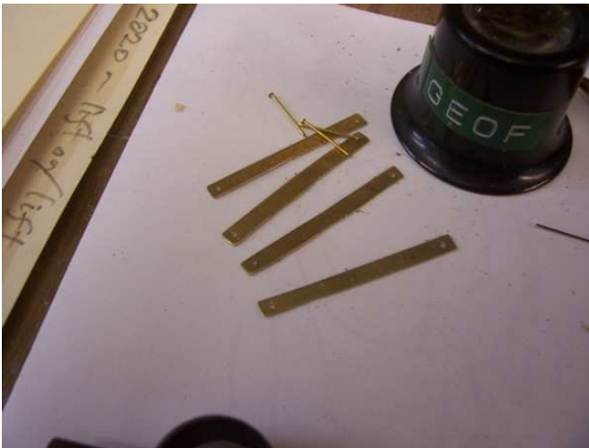
0.5mm x 3.0mm brass braces for posts.
