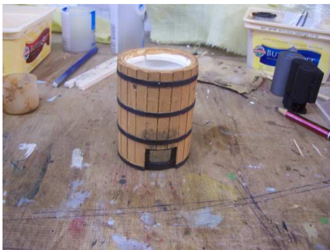
Boiler lagging & barrel bands, holes for feed water, steam pipe, water gauge, wash out plug & fire door.
