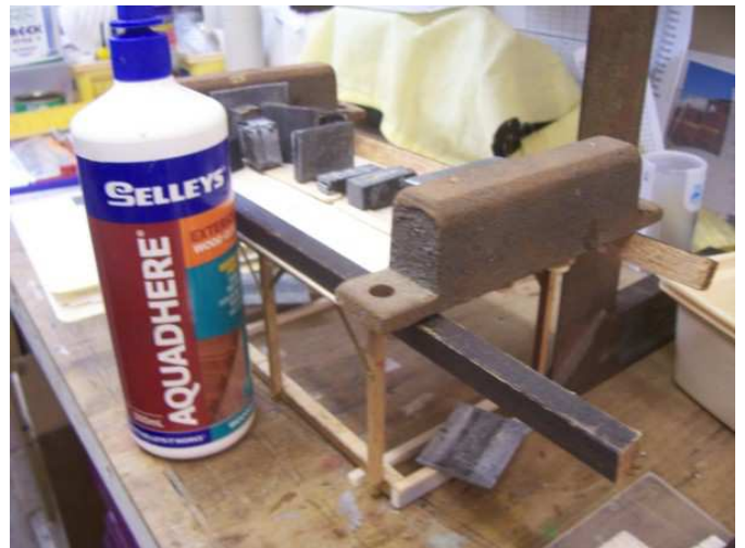
Sides and ends 7 plank 'fences' are glued and drying, roof arc sub strata is glued pressed and setting.
