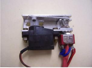
Space was tight for R/C and the standard size Servo with my usual Quadrant Plate that is used to change from Forward to Neutral then to Reverse, so I used a Sub Micro Servo & Conrod throw.
