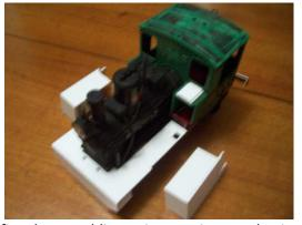
Trial fit sub-assemblies, prior to primer and paint.
