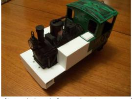
Roof is sanded ready for overhanging new roof.
