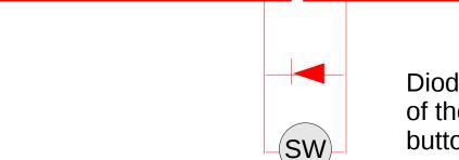
Diode allows locomotive to move out of the siding, pushing the push-button switch allows locomotive to move into the siding. This technique was used to prevent trains from driving off the staging yard. Gaped section must be longer that train length, otherwise you can still back a train off the siding until the locomotive gets to the gap!
