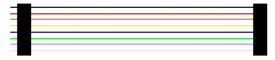
8-pin Cinch-Jones connectors. Male of east end, female on west end. All wires run straight all modules. Track is electrically gaped with insulated rail joiners between modules.
