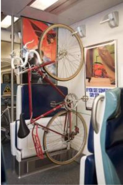
*Metro-North test of bike hook system. Carrying two bikes would lose seating for four passengers.*
