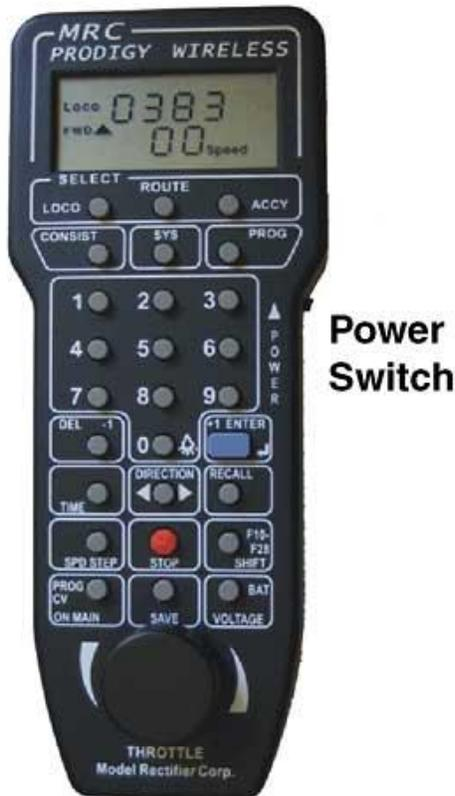
Throttles - A typical throttle display is shown. It provides the engine number, direction, speed, scale time, and which functions are turned on.
