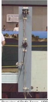
Rear view of Radio Tower. UR91 is at top and UP3 in the middle. Tower is clamped to module and skyboard. Cables run to Command Station and wall-wart.
