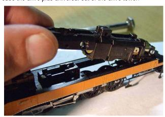
Now remove the skirt assembly by lifting the rear of the assembly while wriggling the front of the assembly over the light tower.
