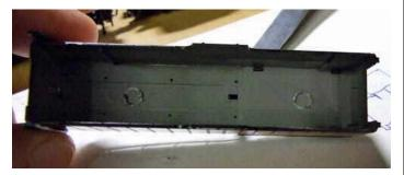
☐ Then cut down the weight cradle so the speaker assembly can be fitted. I also removed about 3/4 of the metal weight.
