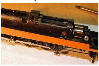
Remove the front light board then lift the front of the upper frame first then gently lift the rear, sliding the upper frame forward. It should separate from the lower frame quite easily. You will also find that the tender will disconnect from the loco. Remove the drive worm retaining clip, then gently ease the drive plus universal out of the drive tower.
