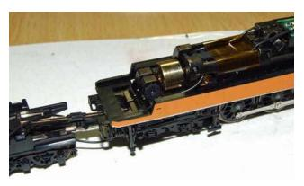
I am utilizing the original Kato analog power board in the tender to transfer track and motor power to the decoder. The first thing to do is drill out the 2 holes in the board. This is to cut continuity from the lower traces to the upper. The next thing to do is to file 2 notches in the forward portion of the board to allow the track pick up wires to thread through.
