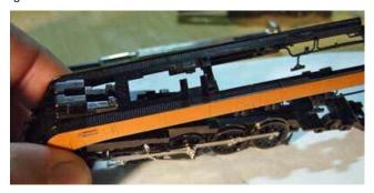
□ You now end up with the upper assembly with motor. It's now just a matter of cleaning the driver wells with alcohol, letting them dry and covering the affected areas with Kapton tape. The following photo shows the driver wells with Kapton tape applied.
