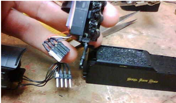
Connector made from computer header pin and plug
