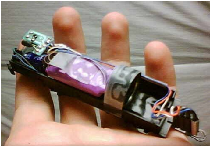
Tender showing installation of SoundTraxx Micro-Tsunami decoder
