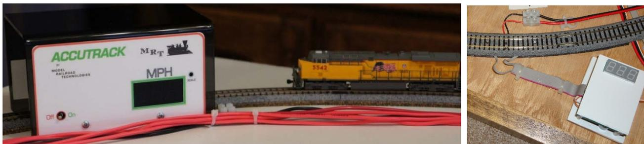
Use of Optional Model Railroad Technologies Accutrack Speedometer or TCS Trainspeed 1 to Verify Loco Speed
