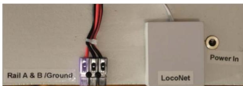
Connections to Command Station + LocoNet + BDL168 Power
