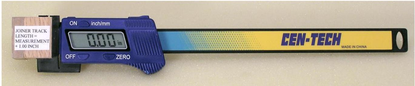
Above is a picture of an easy-to-make gauge that greatly reduces the amount of time it takes us to install joiner tracks at NTRAK meets. This has been used for over 4 years, and it has proven to be very reliable and easy to use.
