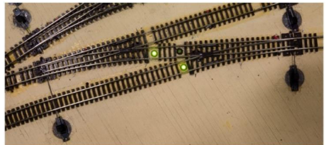
Care must be exercised here because there are two lighted LEDs; one for the Bypass to Track 1, 2 or 3 route and one showing the turnout for the Crossover to track 1, 2 or 3 route although this route is not valid.
