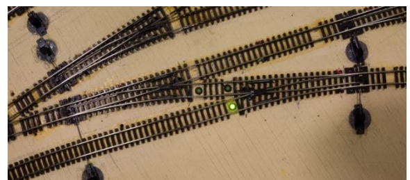
Don't be fooled by this condition. Although the LED is illuminated showing the Crossover route is selected rather than the Bypass, the second LED is dark meaning the route from track 4, 5, or 6 to the Crossover is selected.
