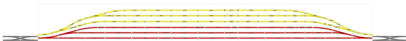
Track Plan for John M Wallis Yard showing Crossover turnouts at each end.
