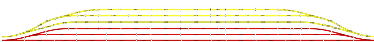
Track Plan for John M Wallis Yard showing red (outer) tracks and yellow (inner) tracks Lowest track for each color is the mainline.
