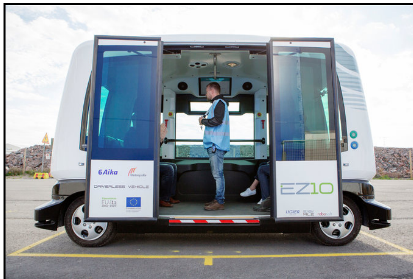
The interior of one of Helsinki's autonomous buses. There's no steering wheel.
