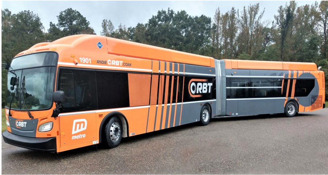
The first ORBT 60-foot articulated bus powered by CNG manufactured in Alabama. (Photo: O-Metro)
