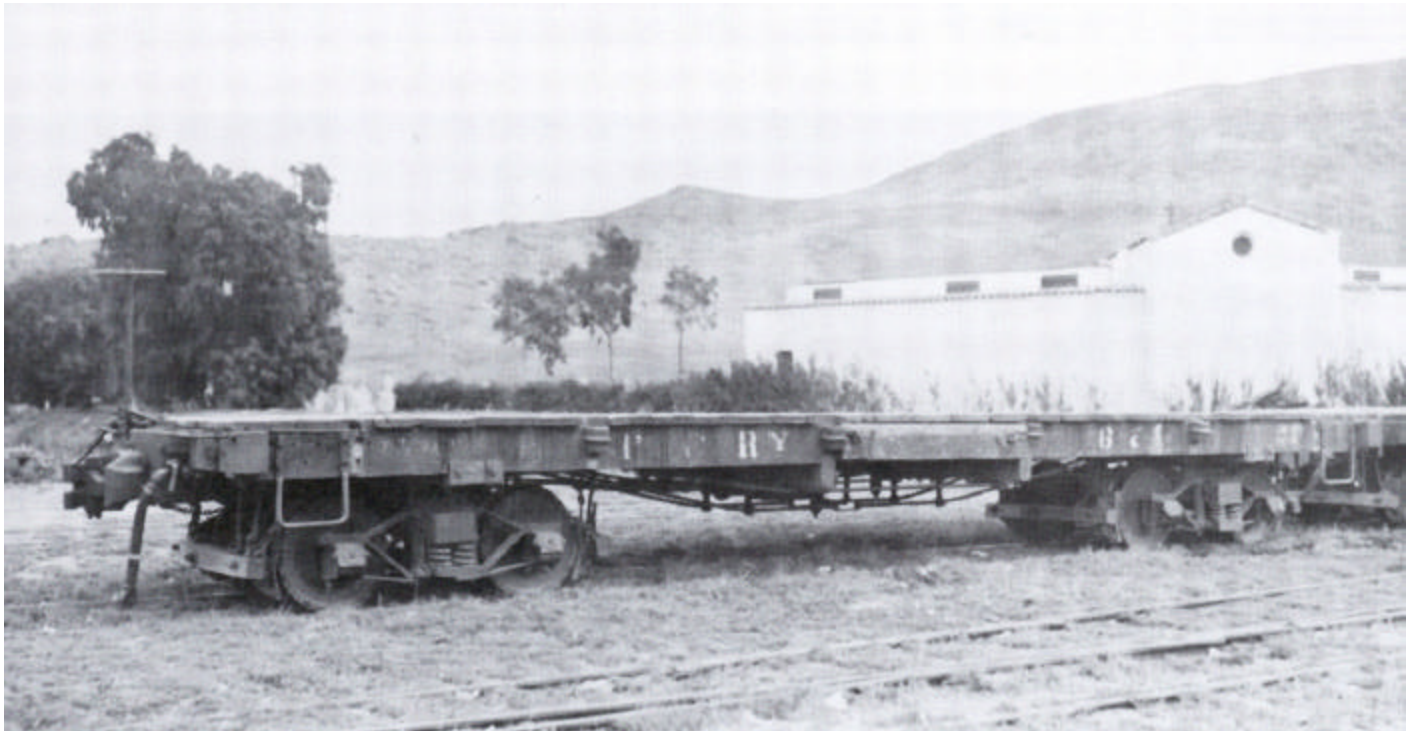
Figure 3. Flatcar #679 at San Luis Obispo, a typical Carter Brothers flatcar except for the step at the center which allows it to be converted to a stock car. The flatcar is backed by the San Luis Obispo Catholic mausoleum at the cemetery near Beebe Street. Credit: Gerald M. Best.
