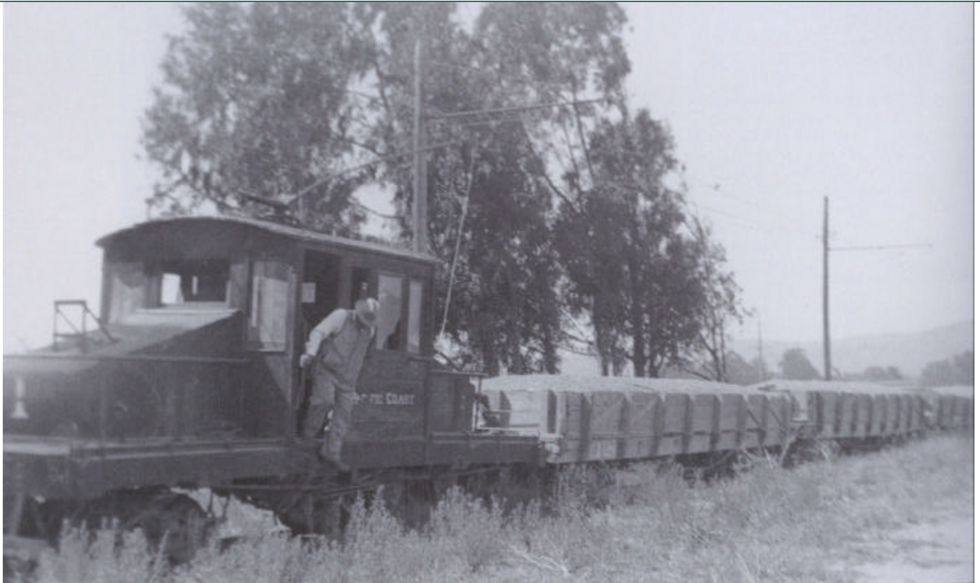
Figure 6. Narrow gauge under wire. Locomotive E-1 on the Betteravia branch. Photo from the collection of Vernon Axt, courtesy of Richard
