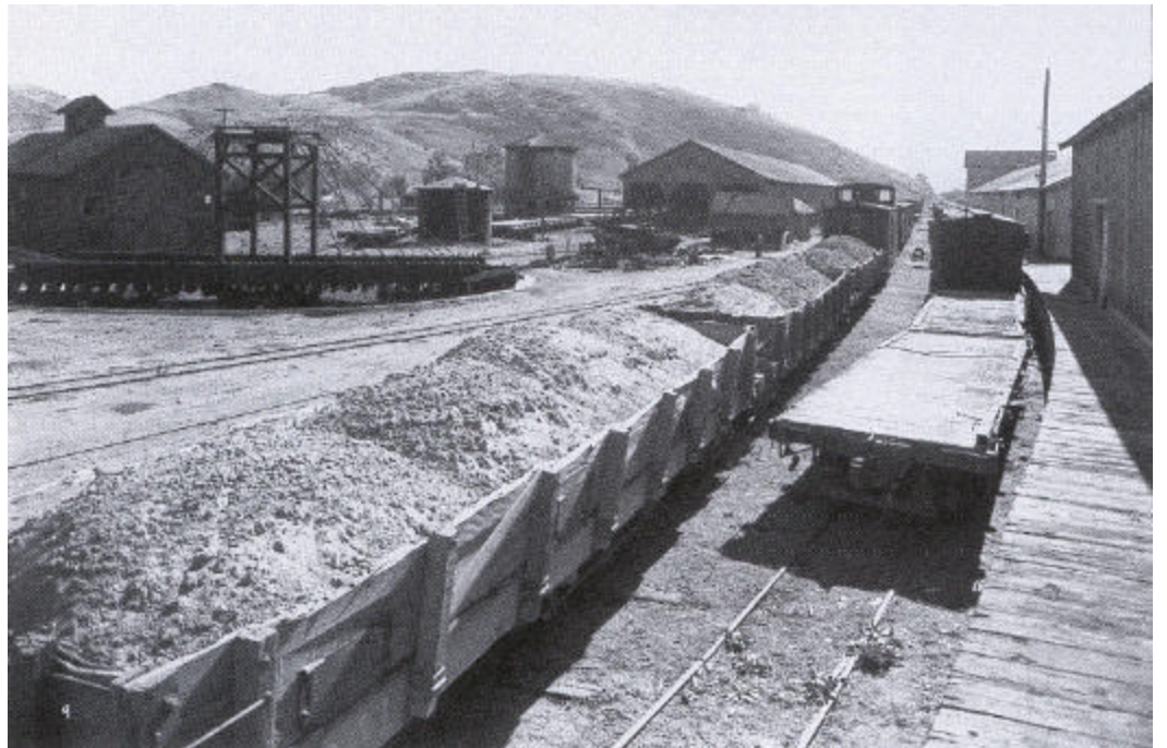
Figure 1: A trainload of sand from Avila arriving at San Luis Obispo in 1939. Note the diagonal bracing and small metal doors on the gondola at right. Young Louis Collection, courtesy of Bennett-Loomis Archives. (Published in The Pacific Coast Railway by Kenneth E. Westcott and Curtiss H. Johnson from Benchmark Publications)
